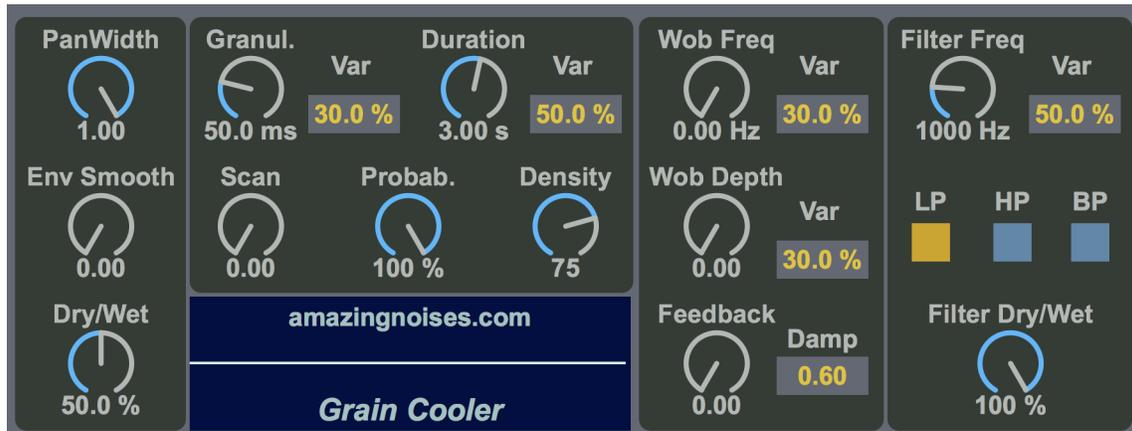
**Grain Cooler** generates polyphonic streams of short grains. Each stream contains a frozen or stretched granulation of the input sound.
