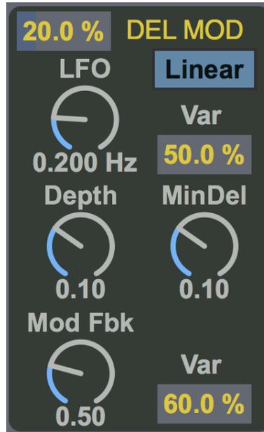
This section shows the parameter for the Delay Modulator effect. The audio input is routed in an LFO controlled variable delay.
