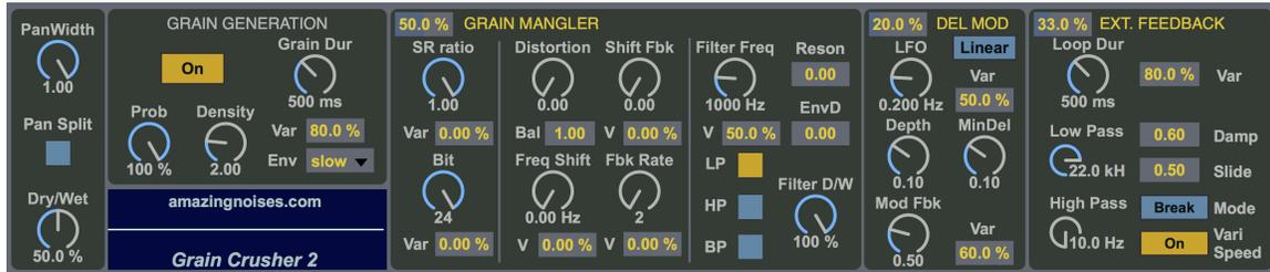
**Grain Crusher 2** is a Max for Live device which performs "Extreme Grain Manipulation". It is a noise and glitch FSU audio effect: you can get a lot of strange and unique sounds from its 3 processing modules: the Delay Modulator, the Grain Mangler and the External Feedback Loop.
